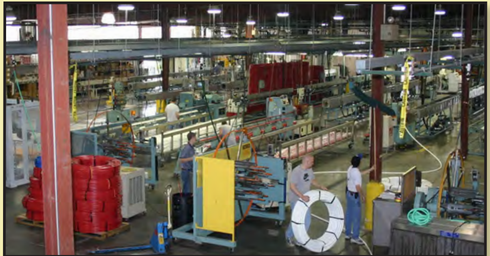
Viega LLC’s PEX extrusion capacity will expand dramatically with the construction of the new manufacturing and logistics facility. This photo shows the primary extrusion operation in the current McPherson manufacturing plant.
